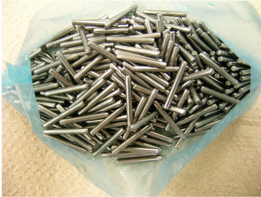
Needle Rollers in 2-mil Cortec VpCI-126 Blue Film (After)
