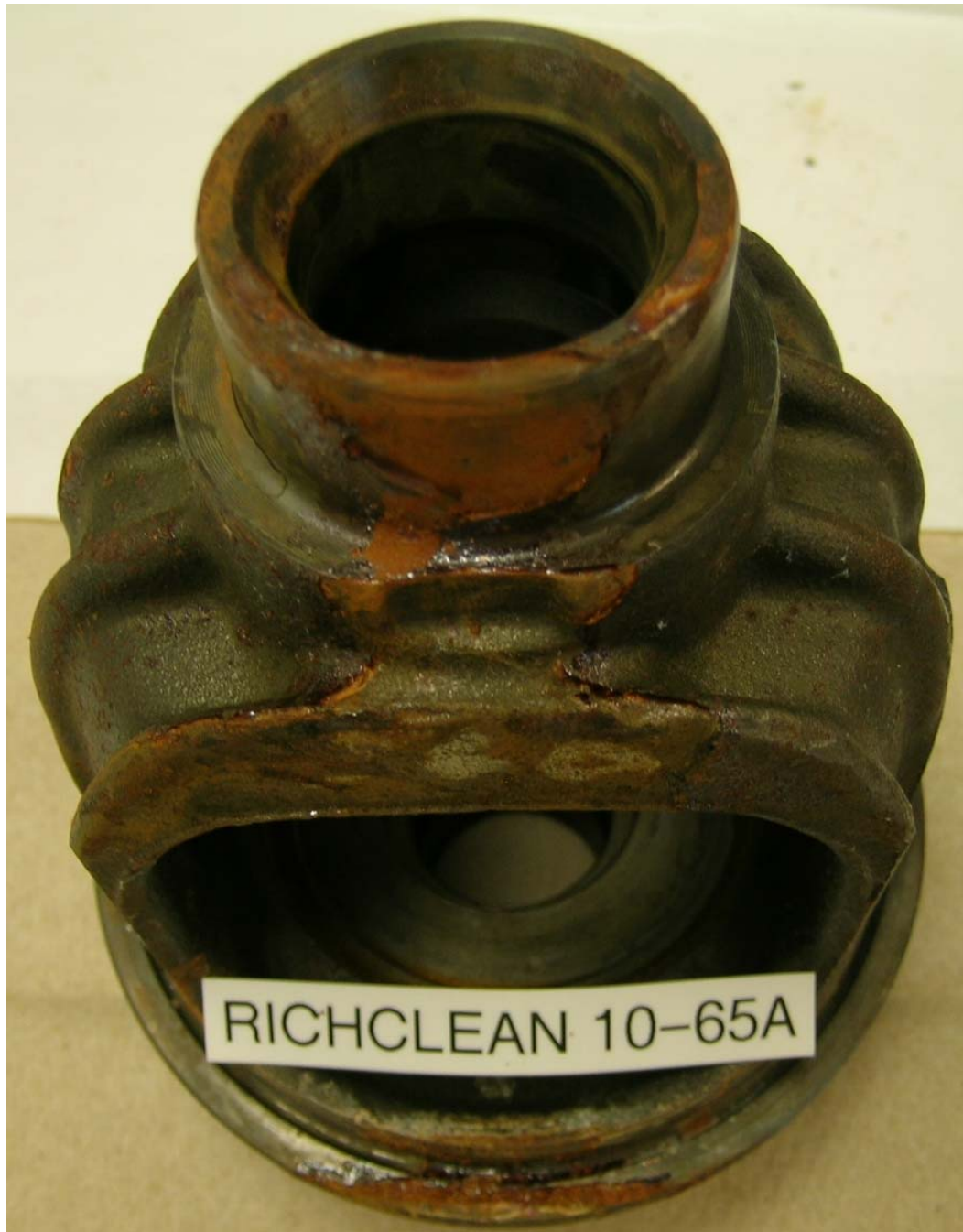
Part dipped in 10% Richclean 10-65A, after 336 hours in ASTM D-1748 humidity cabinet.
