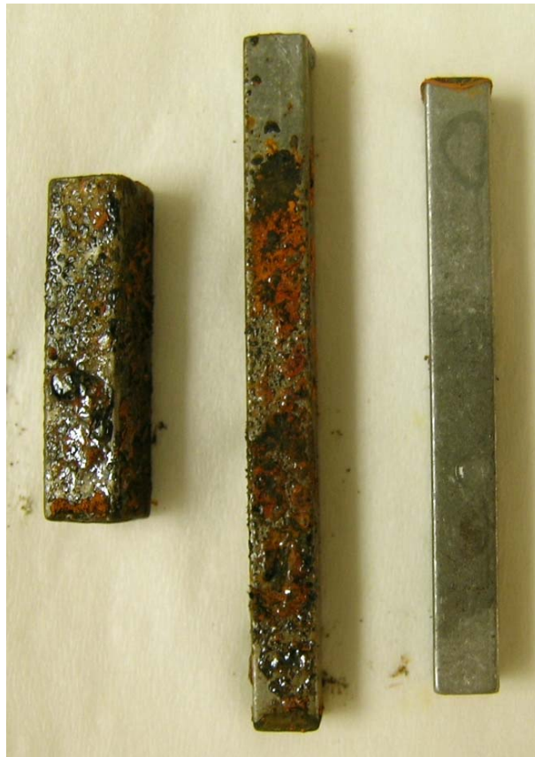
Figure 1: Three keyways after 312 hours in ASTM D-1748 Humidity cabinet testing. From left to right: control, Metal Seal, VpCI-345.
