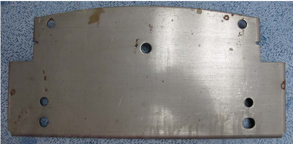
Figure 2: Customer piece coated with VpCI-377, after 500 hours of ASTM D-1748 humidity testing.
