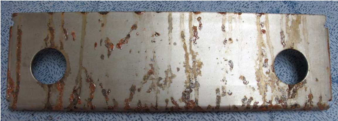
Figure 1: Customer piece coated with DuBois 103SW, after 500 hours of ASTM D-1748 humidity testing.
