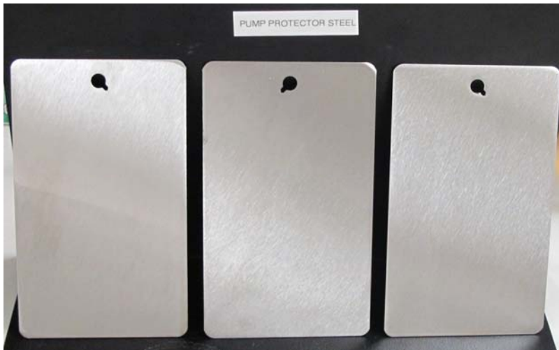
Figure 2. Panels that were coated with EcoLine Pump Protector after being in the humidity chamber for 67 hours.
