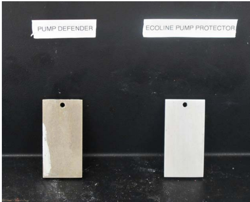
Figure 3. Universal Pump Defender and EcoLine Pump Protector on cast aluminum, after being in humidity chamber for 44 hours.
