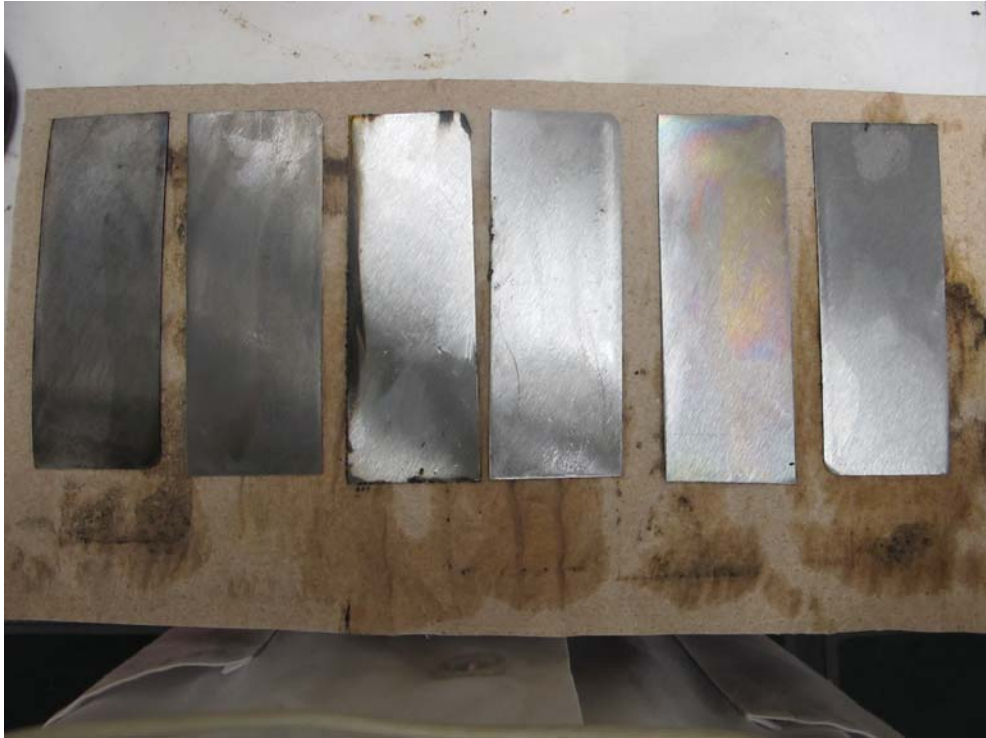
Picture 1: Aligned from left to right are panels 1-6 after being submerged for 216 hours
