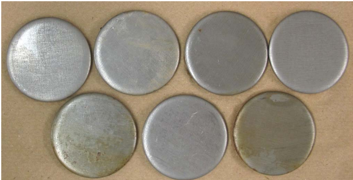
Figure 2: MPI Parts after 500 hours of ASTM D-1735 testing. Products are the same as above, with 3% M-529. The final part on the bottom right was treated with BioCorr.
