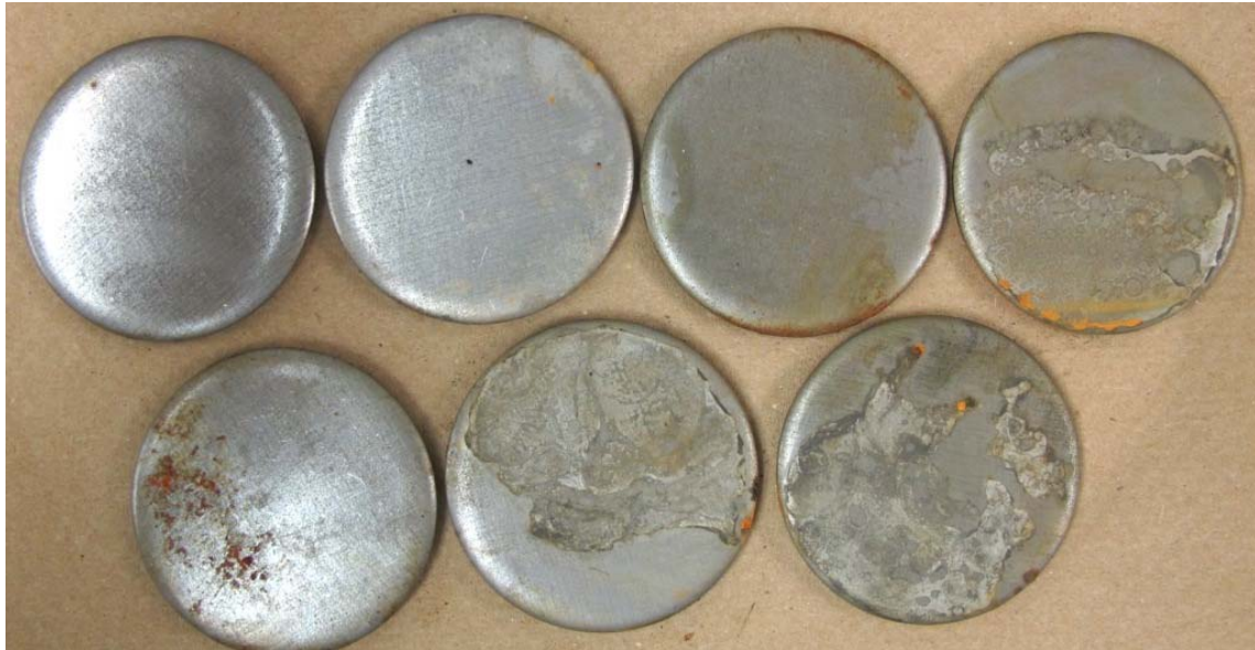
Figure 1: MPI parts after 500 hours of ASTM D-1735 testing. Top row, from left to right: FB-349, FB-485, FB-367, FB-384. Bottom row, L-R: FB-756, RO-7, Inprotect 600
