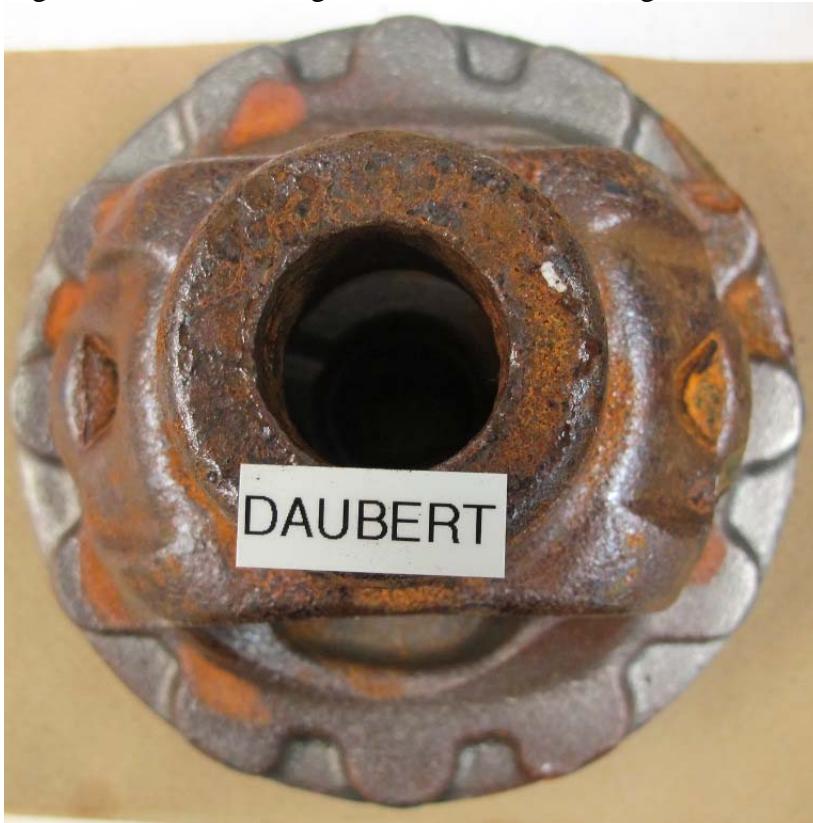
Figure 2: Daubert wrapped casting after 168 hours of testing.
