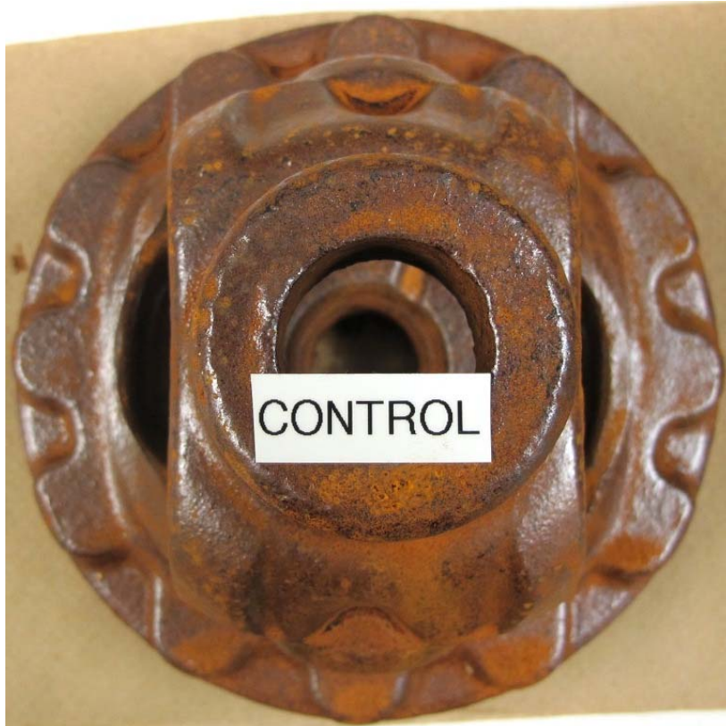
Figure 1: Control casting after 168 hours of testing.
