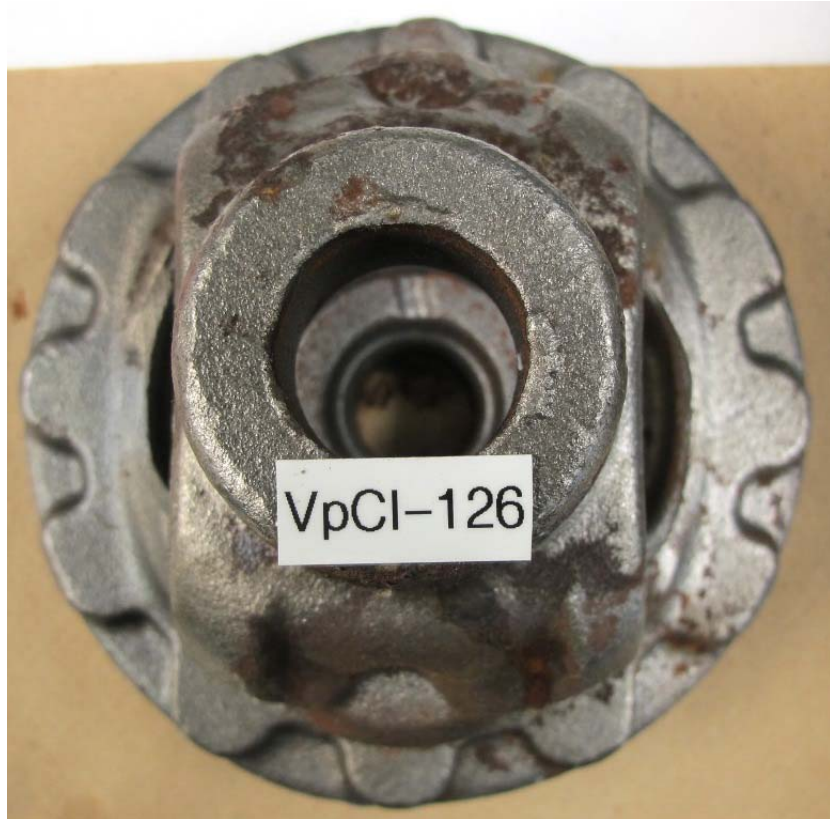
Figure 3: VpCI-126 wrapped part after 168 hours of testing.
