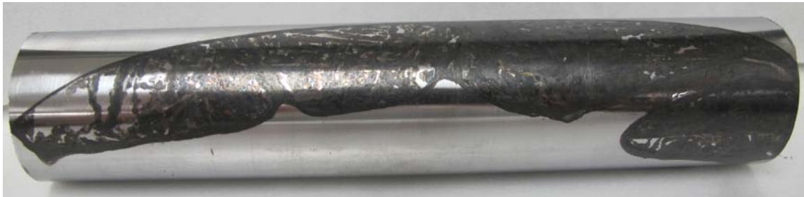
Figure 1: No Rust Preventative (Control)
