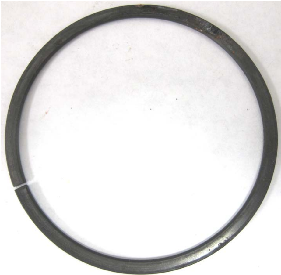
Figure 1: International Chemical 152 coated part after 600 hours of testing
