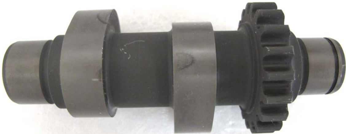
Figure 5: Part 3 protected with VpCI-325
