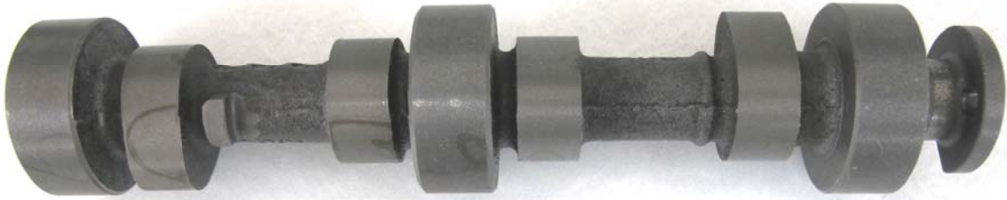
Figure 1: Part 1 protected with VpCI-325
