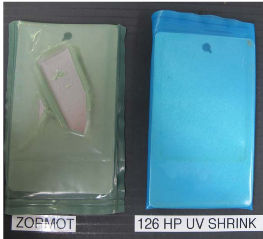
Figure 1. Zormot film and VpCI-126 HP UV Shrink film after being in the QUV for 156 days.
