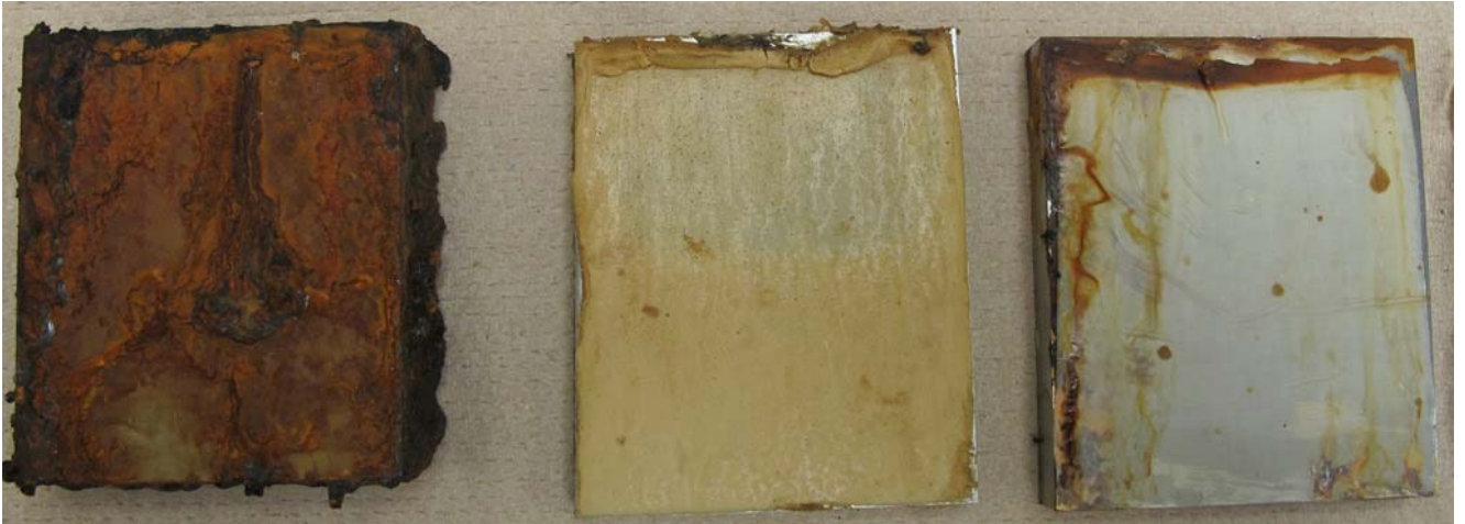
Figure 1: Steel plates after 600 hours in ASTM B-117 salt fog testing. From left to right: Tectyl 506, VpCI-368D, VpCI-389D.
