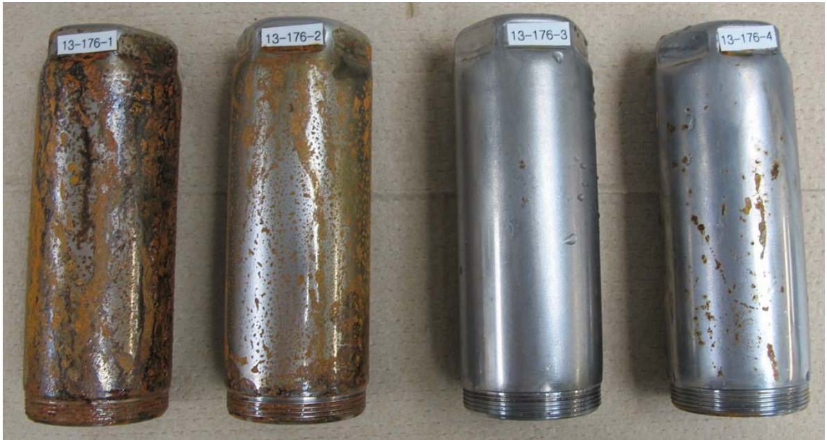
Figure 1: Steel stampings after 500 hours in ASTM D-1735 water fog cabinet. From left to right: Control, Current System, BioCorr, and VpCI-377.
