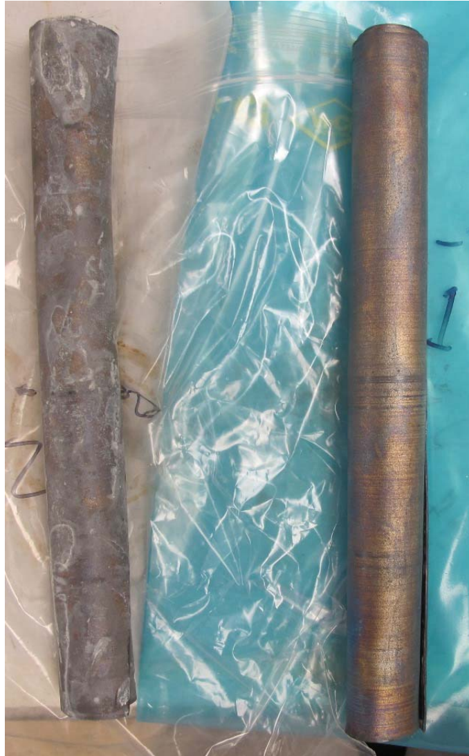
Figure 1: Lead coils after 1000 hours of ASTM D-1735 testing. Non-VCI PE on the left, VpCI-126 on the right.
