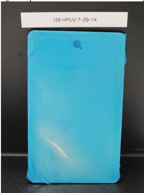
Figure 4. VpCI-126 HPUV films that failed after 158 days in the chamber.
