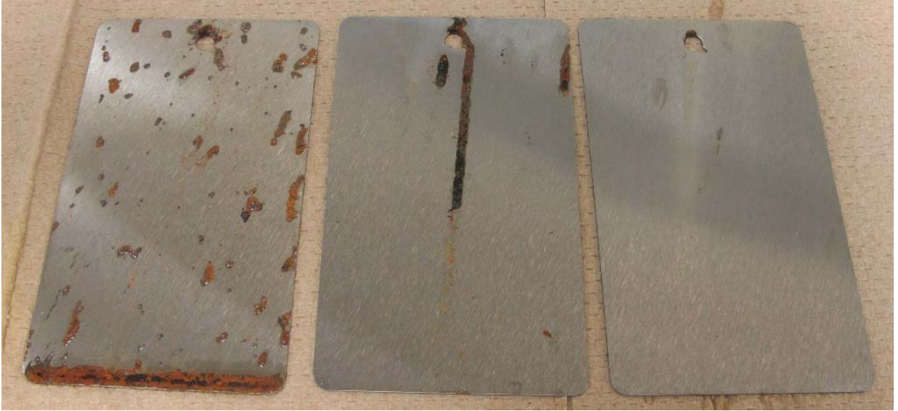
Figure 1: Carbon steel panels, after 480 hours of ASTM D-1748 testing. From left to right: Control, Nox-Rust VCI-10, M-531.
