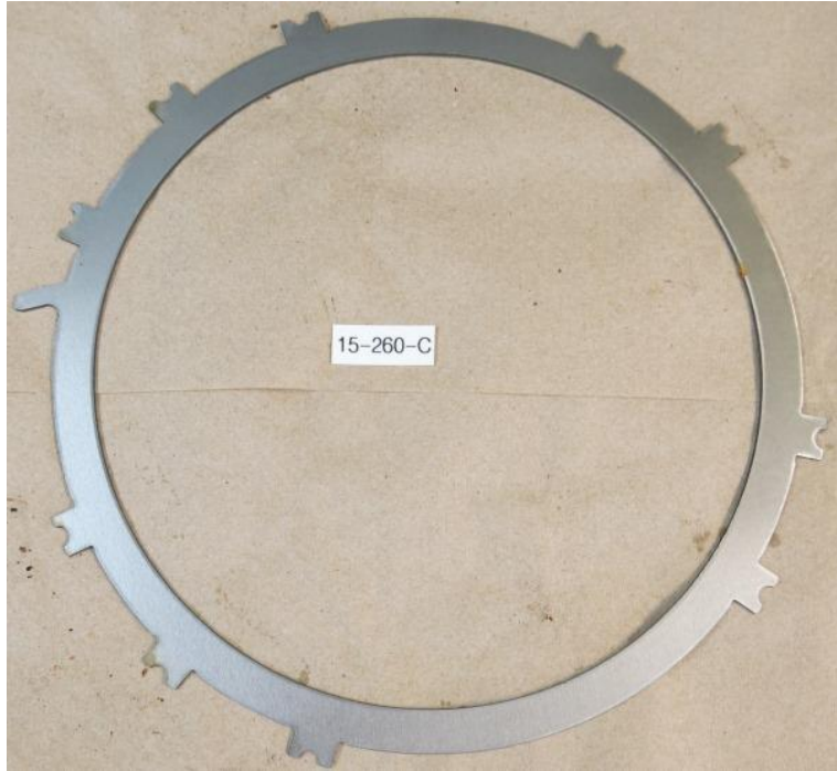
Figure 3: VpCI-325 treated clutch plate, after 624 hours of testing.
