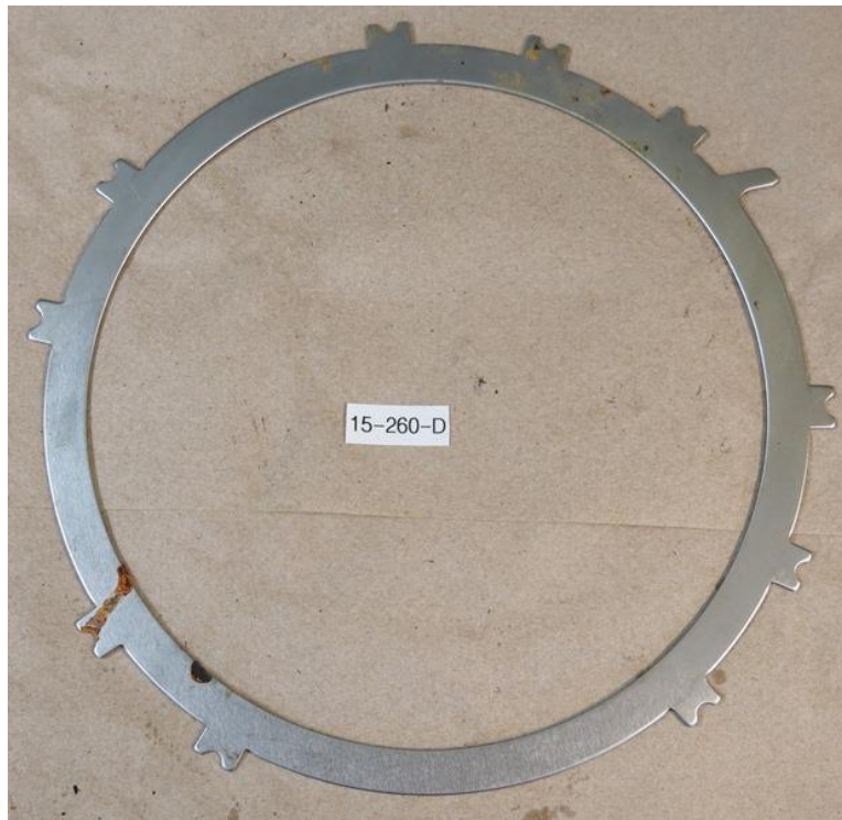
Figure 4: VpCI-329D treated clutch plate, after 624 hours in testing.
