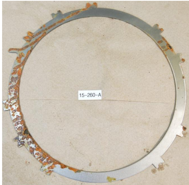
Figure 1: Control clutch plate, after 624 hours of testing.
