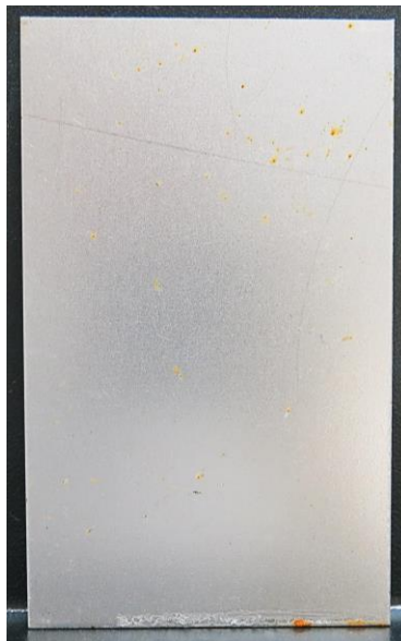
Figure 1: Steel panel coated with Eco Pro after 24 hours of humidity testing.
