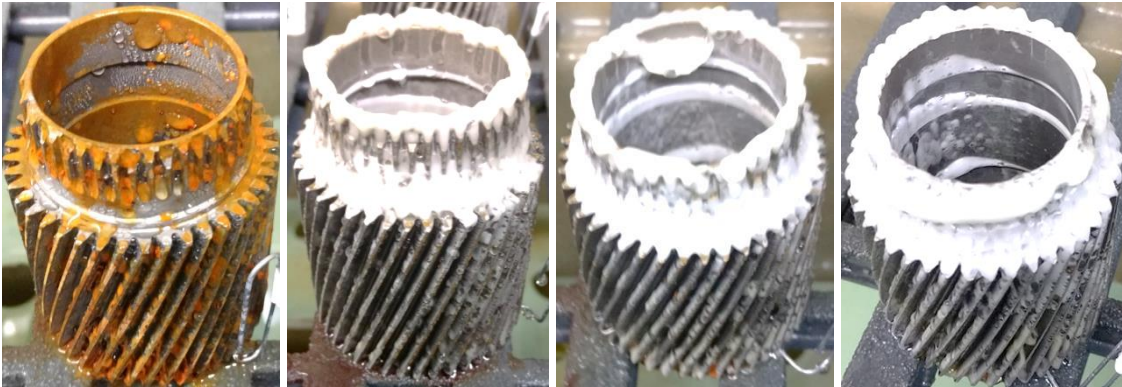
Picture 1: Control sample (left) and Ferrocote rust preventative (three right) at the time where failure was first observed.
