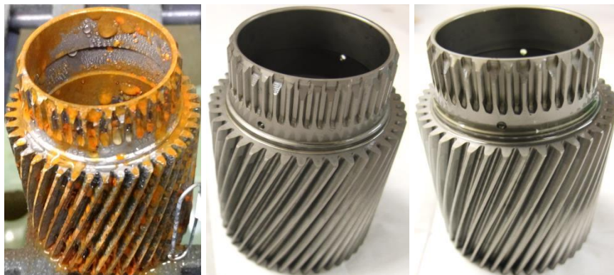
Picture 3: Control sample (left) and VpCI-277 (two right) at the time where failure was first observed.
